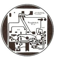
Time-proven etched metal circuit boards are employed in the V-7A. These not only simplify assembly and cut construction time in half, but they permit levels of circuit stability not possible with ordinary conventional wiring methods.
